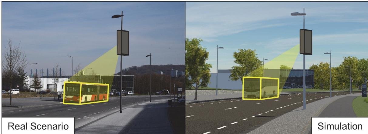
Fig. 4 Design of the digital twin based on a real scenario.
