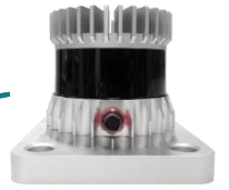
2 LiDAR sensors (128 vertical layers)
